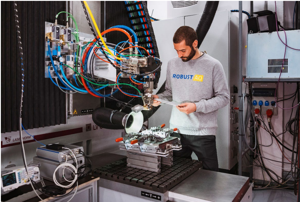
Figure 6, "Zwobbel, beam, shaper, installed, on, a, machine" 3
